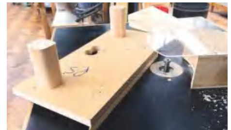
▲ Pic.8 On all components, I planed the outer edges by hand, then using a jig and router, the inner edges where the components meet, to ensure the angles were absolutely spot on
